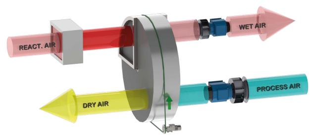
The adsorption dehumidifiers using a technology based on the use of materials naturally drying (ie endowed with high physical-chemical affinity towards water vapor), as the silica gel. This operation technology makes them suitable for use in environments where they are required humidity values even at low temperatures and constant values dew point very low (up to -60°). With this technique it is possible to dehumidify dehumidification any type of environment in any condition.
